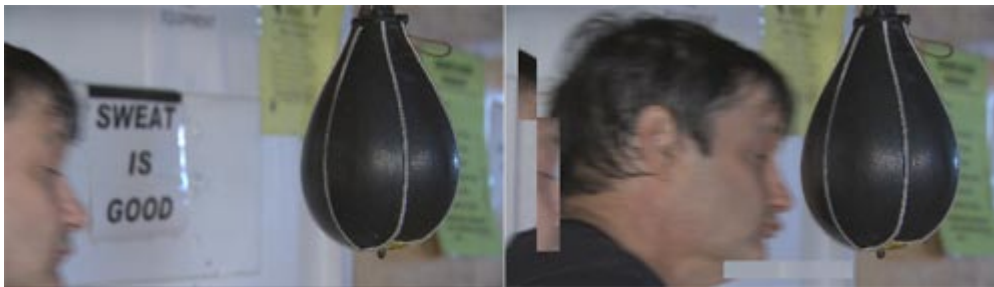
Figure 1: Transmission Error with Concealment on the Right
