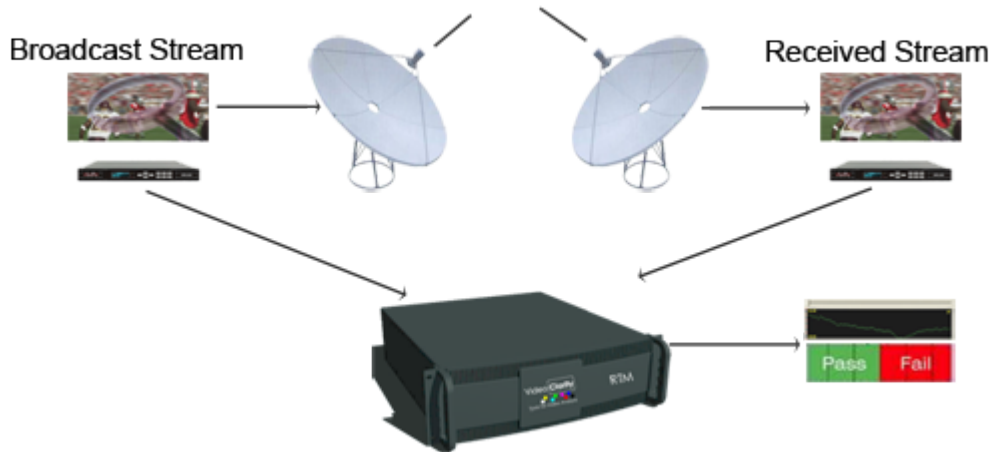
Figure 3: RTM – Monitoring Broadcast OTA compared to Retransmitted Received Signal
